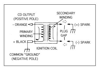
winding and flows only in one direction. The coil fires both spark plugs at the same time; one plug fires from positive to ground, and the other plug fires from negative to positive.
