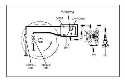
The basic operation of the T-7 C.D.I. system is similar to a conventional C.D.I. system, except with some modifications to include the electronic ignition advance, engine overheat protection, and engine over-rev functions.
