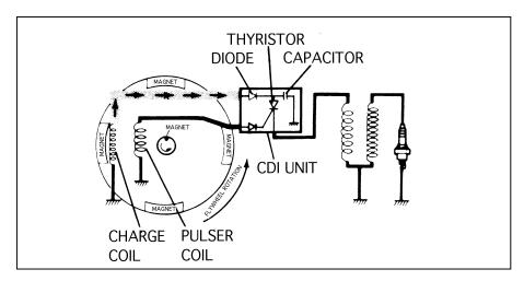
The A.C. voltage is directed to the C.D.I. unit, where a diode converts the A.C. voltage to D.C. voltage. The D.C. voltage charges the capacitor in the C.D.I. unit.
