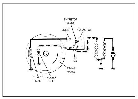
the capacitor, and quickly flows through the thyristor to the primary winding of the ignition coil.
